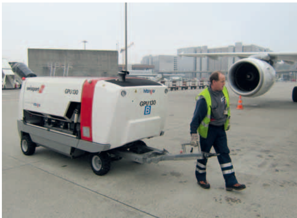
Ground Power Unit
