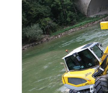
horizontally in the centre part and therefore collisions at the boom cylinder are impossible. The new kinematics of Menzi Muck are also opening up new dimensions: optimum work in the close-up range at the minimum possible swivel radius is contrasted with maximum stretching of the boom. The Menzi power booster thereby supplies the highest possible forces over the whole working range.
